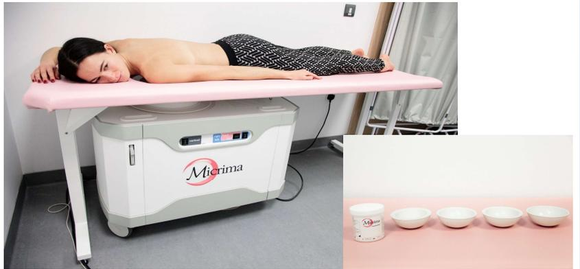
Figure 1(main): Patient (model) positioned on MARIA bed for scanning at Southmead Hospital (inset) Coupling fluid consumable and spacing inserts to accommodate a range of breast sizes.
